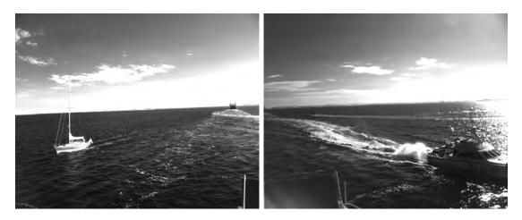
Figure 4.4: Monochrome camera with NIR filter 800 - 1000nm. South Funen archipelago. Ambient condition is daylight and good visibility
