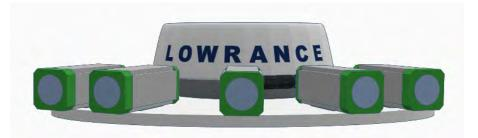
Figure 4.1: Sketch of the sensor platform. The five camera houses are looking forward in the ships heading. Camera units, CW-FM radar and GPS receiver plus IMU are fixed on the platform.
