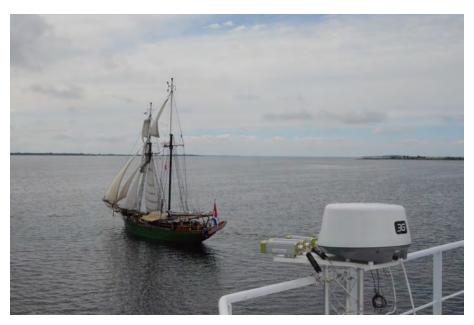
Figure 4.2: Southern Funen archipelago. Sensor platform mounted beyond wheelhouse / ship's bridge.
