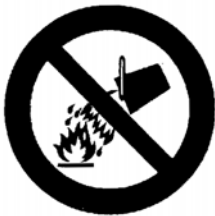
Do not extinguish with water
