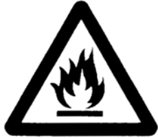
Flammable material or high temperature (1)
