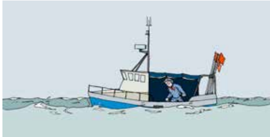
Vessels with low freeboard
